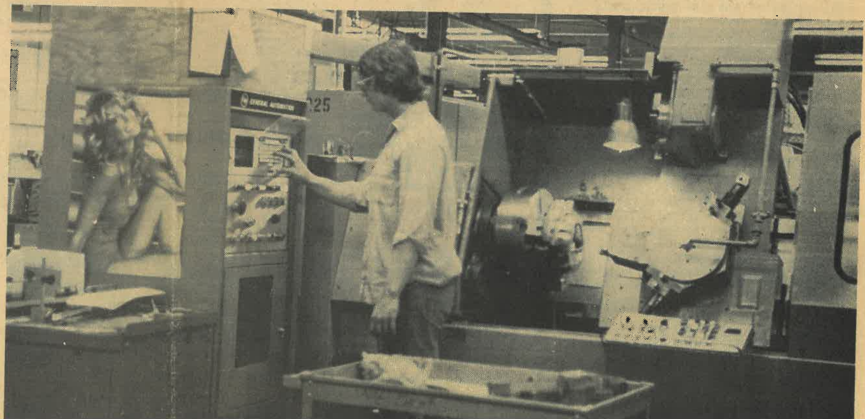
Steve Schultz is operating a numerical control lathe. The machining operation is controlled by computerized tape. Over the last four years, the company has purchased 14 of these machines. Another machining center operation controlled by computerized tape is being done by War- dell Scruggs. Betty Stewart is pictured above operating a Sheldon lathe also computerized. Elizabeth Badgerow is one of the laminated molders working in the fiberglass department. Pictures, in a circular sequence from top right, illustrate some of the different processes which create the finished product.
