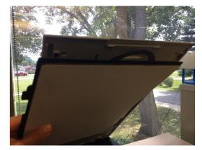
3. Select the appropriate film/slide tray and align the lettered tab on the tray with the matching lettered slot on the scanner so the tray is lying flat on the glass.
