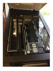
4. Insert the slides/film in the appropriate slot(s) of the tray. The shiny base side should be facing down. Your images should appear backwards on the side that faces up. You can insert 1 strip of medium format film, up to two 35mm film strips or up to 4 35mm mounted slides. Each scan takes approximately 1 minute, 13 seconds.
