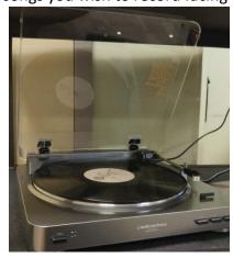
4 Raise the "**Tone Arm**" and move it over the beginning groove on the record. The record player will automatically turn on and the turntable will begin to spin.
