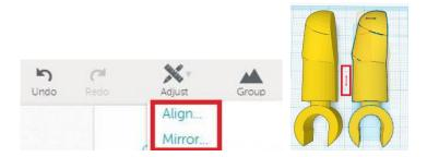
**Step 7:** Clicking on the arrow highlighted above will rotate the selected arm vertically, mirroring the original arm.
