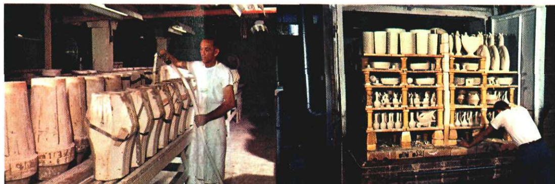
Pouring "slip" to duplicate original design.
